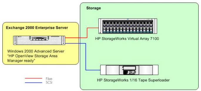
figure 2 - example entry-level Exchange solution physical view
