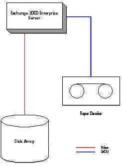
figure 1 - entry-level Exchange solution logical view
