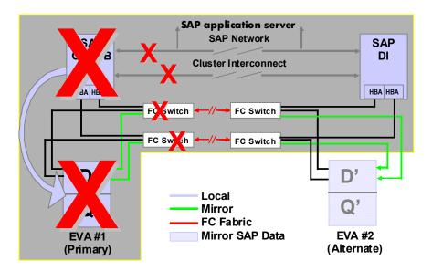
Depending on which Continuous Access management interface is used, the following steps must be taken to complete a site failover for both configurations after the remote HP OpenView Storage Management Appliance has access to alternate site EVA:
