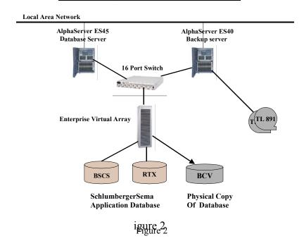
The main solution elements (Figure 2) are described below. A more complete BOM follows in section 3.3.
