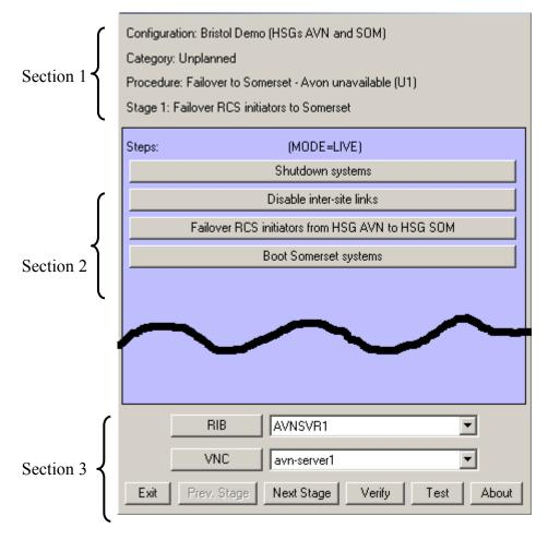
Figure 10 – Recovery Manager – Site Failure Procedure, First Screen
