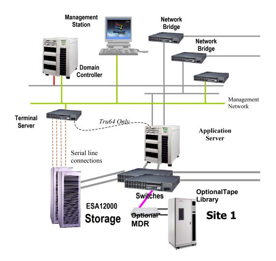
Figure 2 - Diagram showing typical serial connections for active monitoring (single site)
