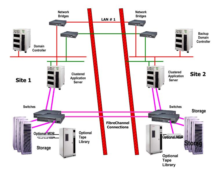
Figure 1 – Example of a basic SAN deployment for the DT-SAN Solution
