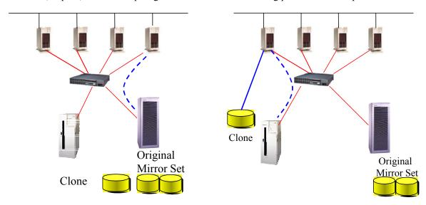
Figure 1: The Cloning Process Before and After Split
