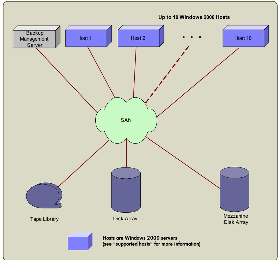
figure 1. mezzanine two-stage backup solution: logical view
