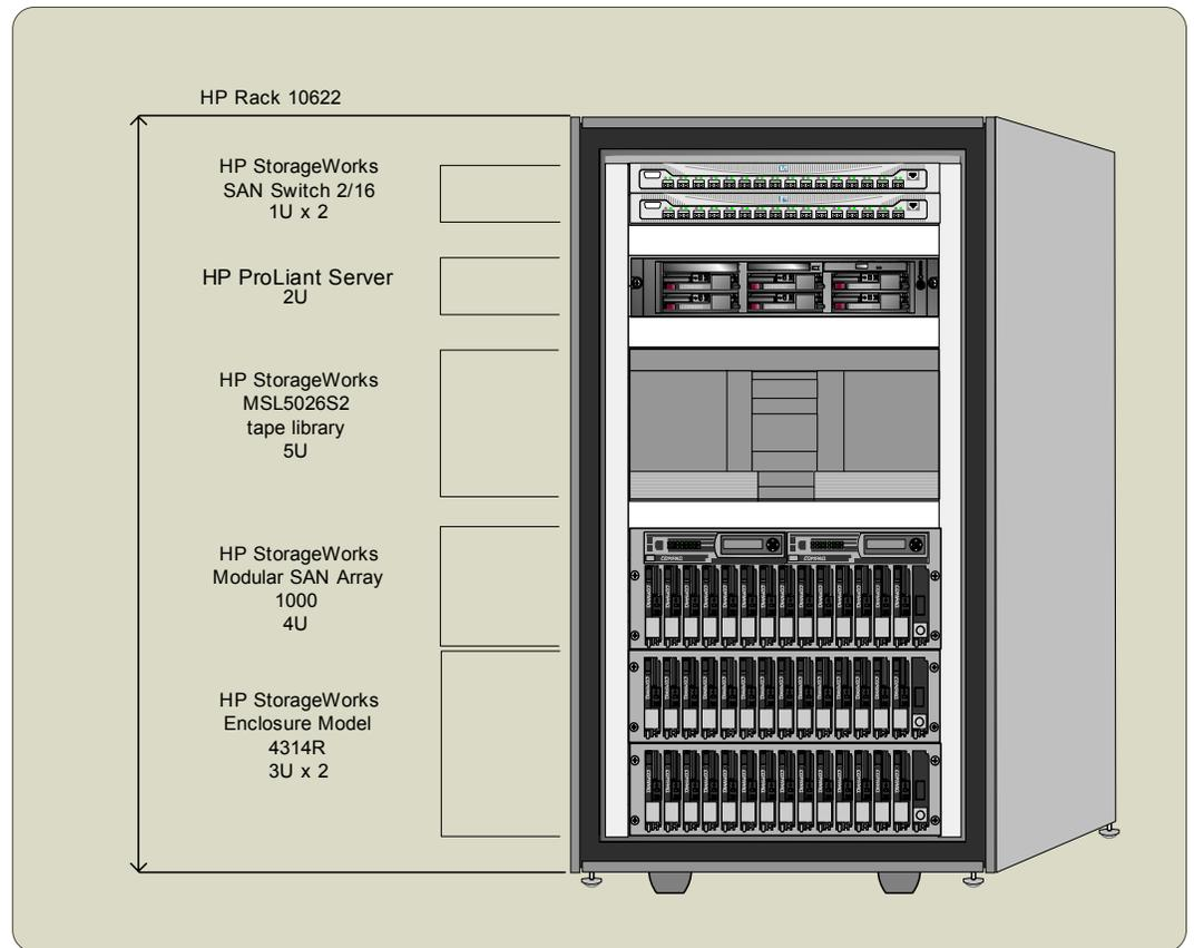
**figure 3. example mezzanine two-stage backup solution rack**
