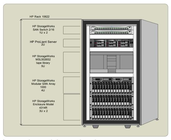
figure 3. example mezzanine backup-restore solution rack
