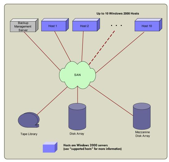
figure 1. mezzanine backup-restore solution: logical view
