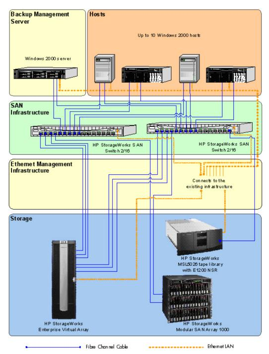
figure 2. mezzanine backup-restore solution: physical view
