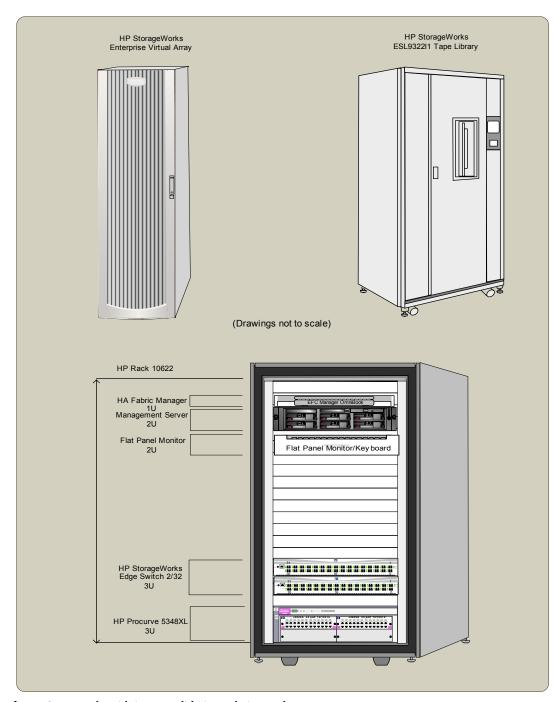
figure 3. example mid-tier consolidation solution rack
