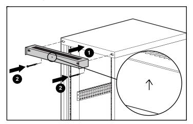
Figure 3: Installing the spacer top assembly
