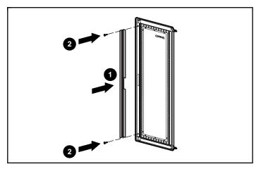
Figure 7: Installing the vertical vented spacer to the door
