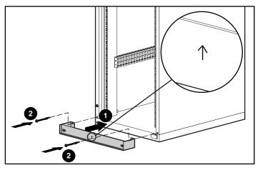
Figure 4: Installing spacer bottom assembly
