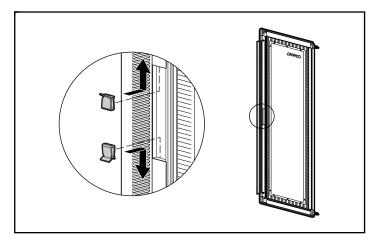
Figure 8: Installing door clips
