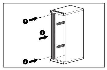
Figure 6: Installing the vented spacer fixed side panel
