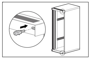
Figure 9: Reinstalling door latches
