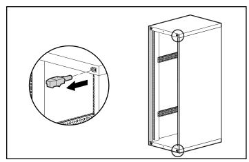
Figure 2: Removing the door latches
