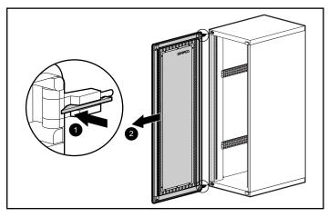
Figure 1: Removing the door from the Compaq Rack 7142
