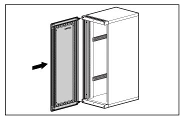
Figure 10: Reattaching the door
