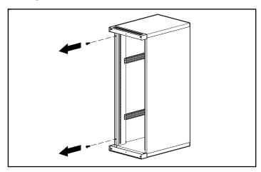
Figure 5: Removing the hinge-side screws
