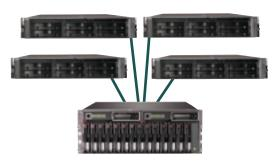
MSA1000 connected to four HP ProLiant DL380 servers via a Fibre Channel switch with Selective Storage Presentation
