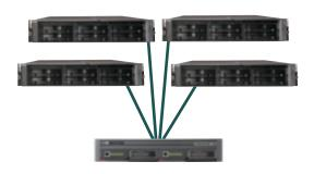
MSA1500 connected to four HP ProLiant DL380 servers via Fibre Channel SAN attached 2U controller shelf with Selective Storage Presentation
