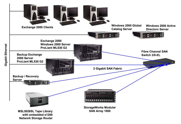
figure 2. DAS-to-SAN Exchange 2000 migration solution, post-migration configuration
