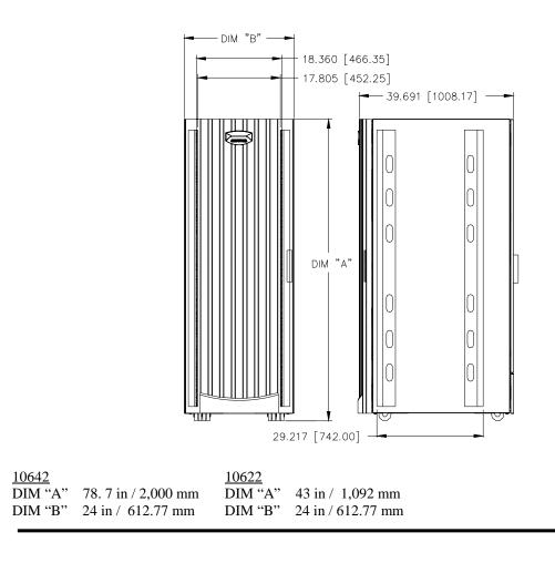
A "U" is the measuring unit for racks and rack-mountable components. 1U = 1.75" or 44.45 mm.
