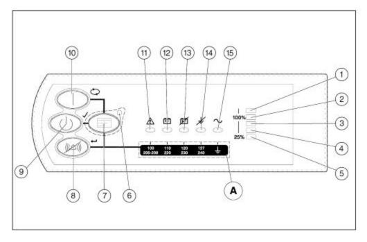
Figure 4: Front Panel of the Compaq UPS R3000 XR<sup>1</sup>
