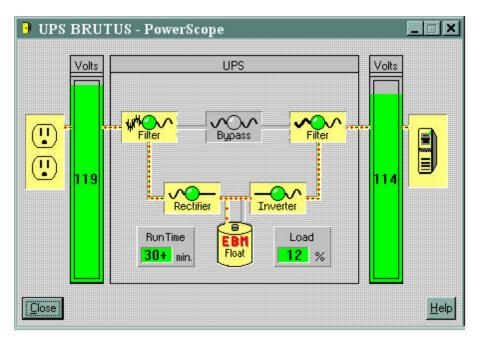
Figure 7: PowerScope Screen
