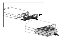
Figure 3: Hot-swappable battery and electronics module
