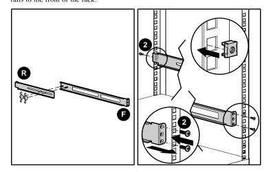
Align the bracket with screw holes in unit. Use screws **1** to attach brackets to sides of unit. Slide unit into rails and secure by using screws **2** to attach unit.
