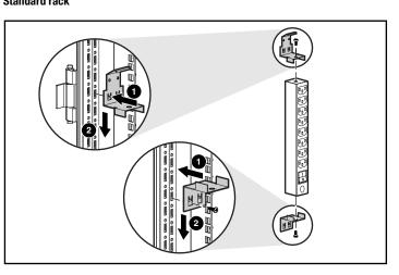
If the bracket interferes in the upper or lower positions in the rack, squeeze tabs, as shown. This view assumes the extension bars are mounted on the left side of the rack. If mounted on the right side of the rack, squeeze the left tab.
