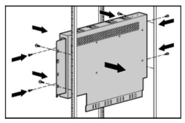
Figure 3: Compaq Dual Input PDU in a zero-U Configuration
