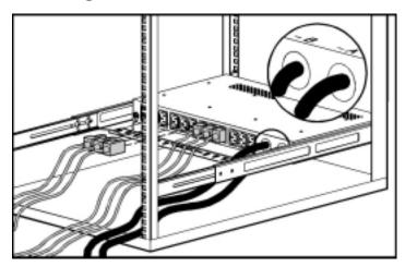
Figure 4. Compaq Dual Input PDU in a 1U Configuration
