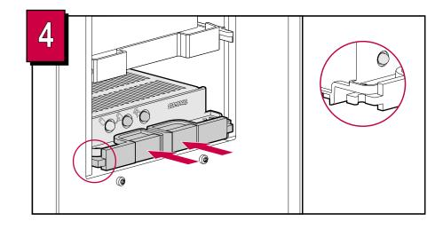
Close the ejector levers behind the front panel of the disk enclosure to complete the installation of the drive.
