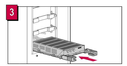
Make sure the ejector levers are in the full open position to ensure a correct latch while installing the drive into the disk enclosure.
