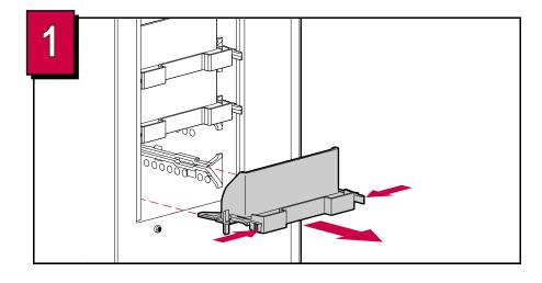
Remove the failed drive or blank drive bezel from the disk enclosure before installing a new hard drive.
