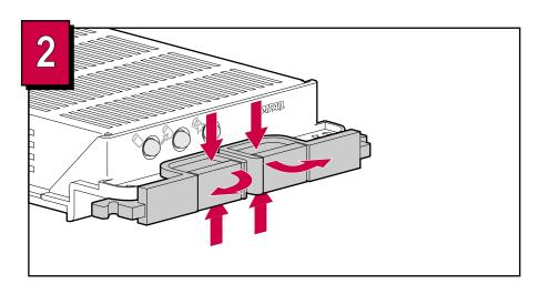
Squeeze the latches and pivot the ejector levers on the drive to the full open position.
