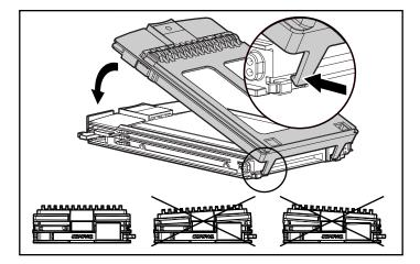
To confirm a correct attachment, the front view should be level on both the right and left sides and the fit should be snug.
