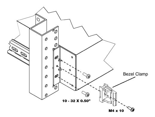
Figure 12 Rear Tie-Down Mounting Detail
