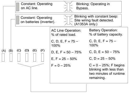
LEDs (A), (D), (E), and (F) are green. LEDs (B) and (C) are amber (yellow.). LEDs (A), (B), and (C) are used to show operating mode or alarm conditions. LEDs (C), (D), (E), and (F) are used to indicate load or remaining battery capacity. An Alarm Condition exists when LED (C) is blinking or when an audible beep is sounding. (Three beeps every five minutes is normal indication of battery charging.)
