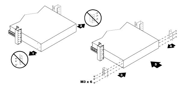
Figure 11 Securing Unit At Front And Mounting Bezel Clamp
