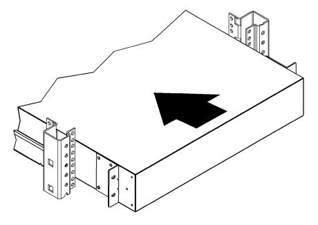
**Figure 7 Securing Units to Front**
