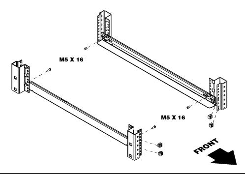
**Figure 6 Mounting Units on Support Rails**
