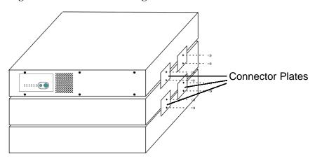
If the HP PowerTrust II-LR UPS is to be mounted on the floor, the A1357A Battery Packs should be placed first. The UPS should be on the top of the stack. The units should be secured together with the HP A1363A Deskside Hardware Kit. Each kit consists of four connector plates and eight screws. Two connector plates should be mounted on each side of a unit to join it to the one below. See Figure 13.
