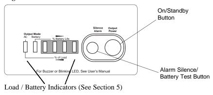
The HP PowerTrust II-LR utilizes six LEDs (Light Emitting Diodes) and an acoustic alarm to indicate various conditions. The Alarm Silence/Battery Test button is used to silence acoustic alarms if they are present. In the absence of an alarm condition, this button is used to initiate
