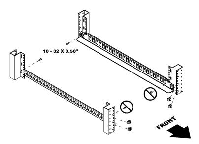
Figure 10 Removal And Replacement Of Mounting Brackets
