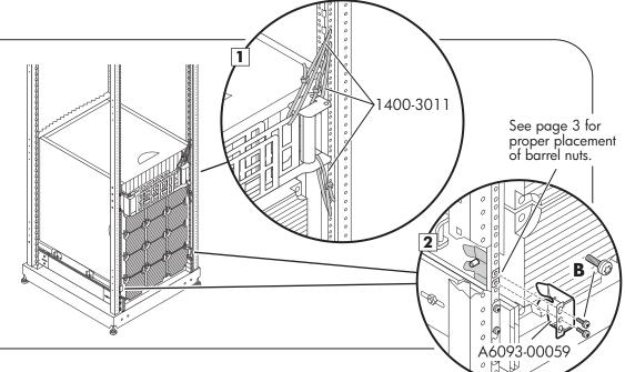
Attach barrel nuts to the front and rear columns as shown in the diagram below. 0 barrel nut (D) NOT TO SCALE 00 0 0**0** 0 PRODUCT OUTLINE PRODUCT OUTLINE 0 16U 16U 15U 15U 117.5 mm (4.63 inch) 1.3 14U 14U <u>ම</u> ි 13U 13U 12U 12U -444.5 mm (17.50 inch) 11U 1.4 11U 10U 10U 9U 9U -431.8 mm (17.00 inch) 17 U <sup>8U</sup> 8U 17 U 7U 6U 6U -5U 5U 165.1 mm (6.50 inch) 4U 4U 3U 3U 44.5 mm (1.75 inch) 0 2U 2U **↑** 73.0 mm 73.0 mm 0 1.2 (2.88 inch) (2.88 inch) 1U 1U
