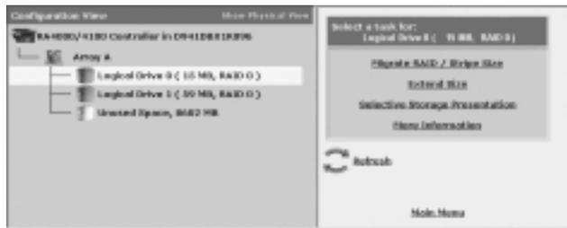
**Figure 2-8: Typical task list for a logical drive**
