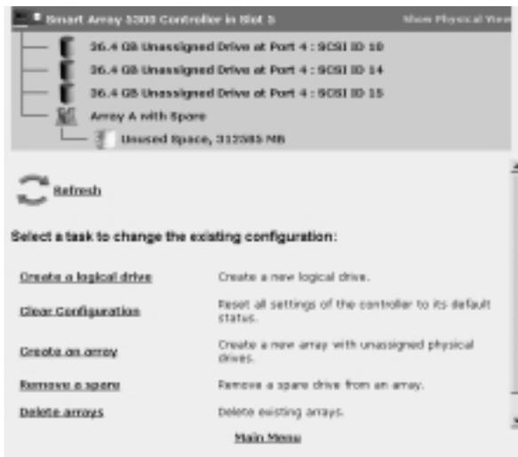
Figure 2-5: Configured array screen (no logical drives)
