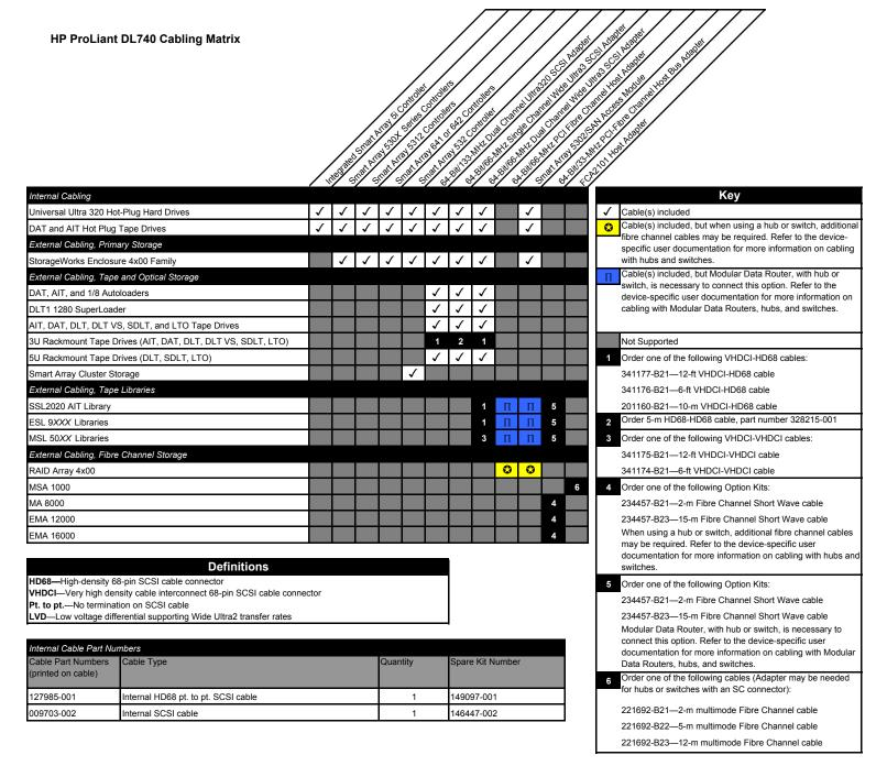
**NOTE:** The information in this matrix lists whether or not additional cables need to be purchased with each controller-to-option configuration. For information on how to cable an option, refer to the *HP ProLiant DL740 Setup and Installation Guide*, the device-specific documentation, and the controller-specific documentation. For information on the specific options supported by the server, refer to the server and device QuickSpecs.
