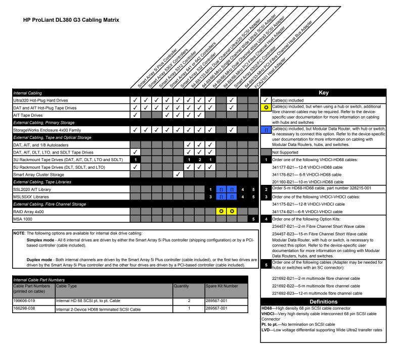
**NOTE:** The information in this matrix lists whether or not additional cables need to be purchased with each controller-to-option configuration. For information on how to cable an option, refer to the *HP ProLiant DL380 Generation 3 Documentation CD*, the device-specific documentation, and the controller-specific documentation. For information on the specific options supported by the server, refer to the server and device QuickSpecs.
