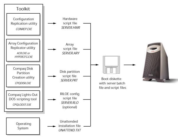
Figure 1-1: SmartStart Scripting Toolkit server deployment process
