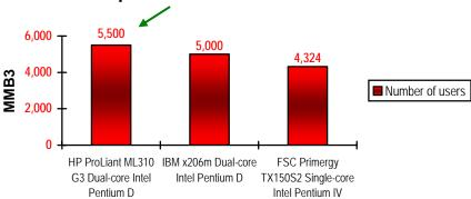
The ProLiant ML310 G3 server achieved an average CPU utilization rate of **84.8**% during the **5,500** MMB3 test, weighted 95th percentile response-time score of **318** milliseconds (s), and average send-queue size of 46 messages for the four-hour steady-state period.
