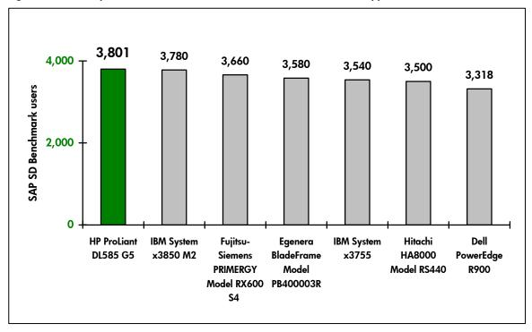
Figure 1. Several 4-processor Windows results on two-tier SAP SD Standard Application Benchmark<sup>2</sup>
