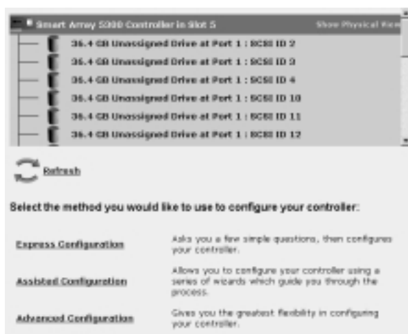
Figure 2-1: Starting to configure a new controller
