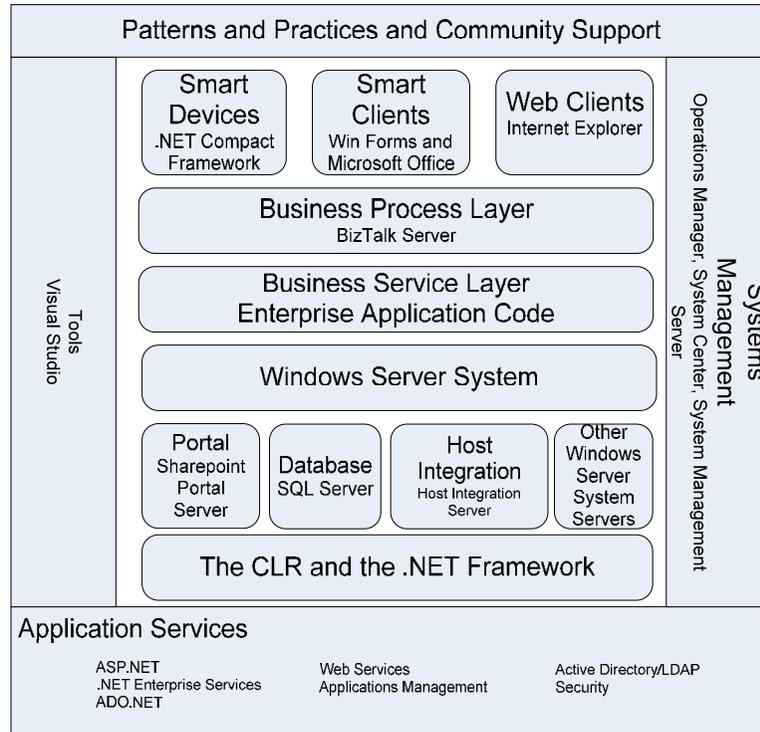
**Figure 2: The Microsoft Enterprise Application Development Platform Core Technologies and Products**
